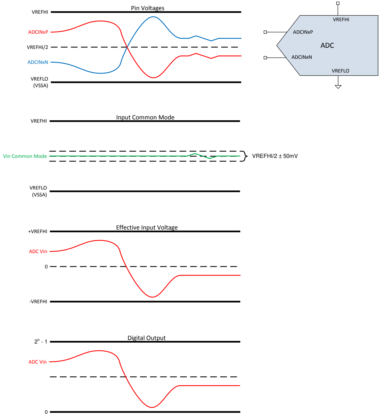
Figure 8-31. Differential Signaling Mode
